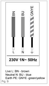
This appliance is intended to be connected to fixed wiring by a double pole switch, having a contact separation of at least
